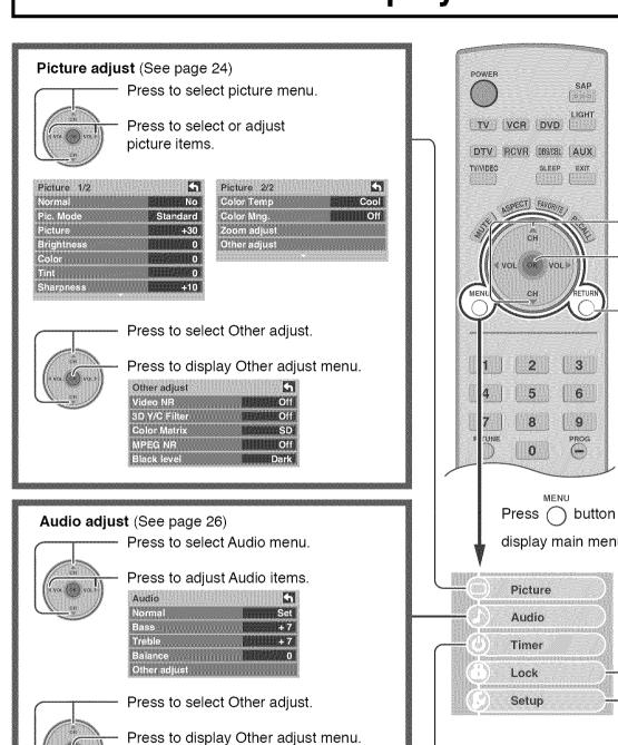
Press to select. Press to enter each adjust screen. Press to return to previous menu. Press ( ) button to display main menu.
