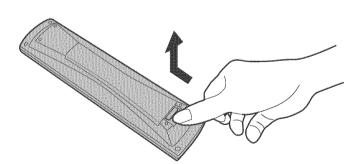
Install the batteries and replace the cover.
