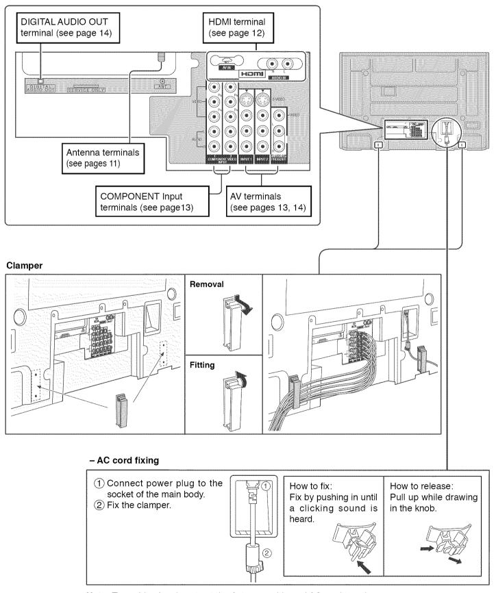
Note: To avoid noise do not put the Antenna cable and AC cord together.
