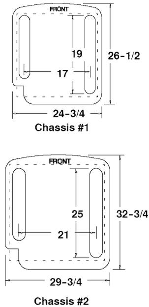
Minimum Mounting Pad Sizes with pad starting at 15" from structure for minimum clearances
