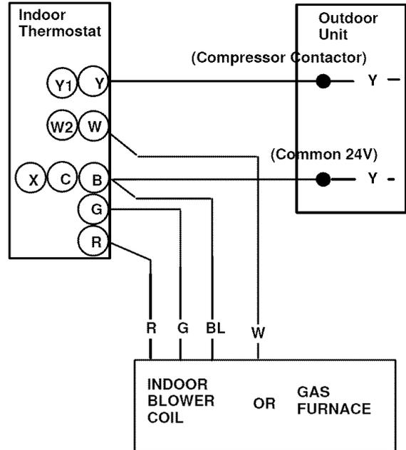
**Figure 11** Heat Pump Typical Low Voltage Control Connections
