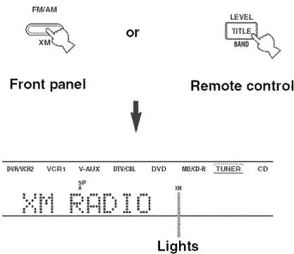
If "CHECK ANTENNA" appears in the front panel display, the XM Connect and Play digital antenna accessory may not be connected to the XM jack on the rear of this unit properly. See "XM Satellite Radio connections" on page 44 and check the connection.
