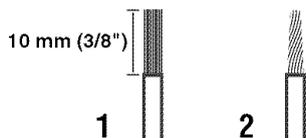
**1** Remove approximately 10 mm (3/8") of insulation from the end of each speaker cable.
