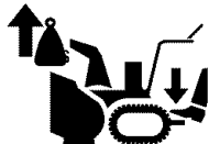
Weight Transfer Depress Pedal To Disengage
