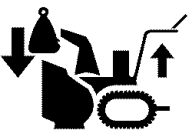
Weight Transfer Lift Handle To Engage
