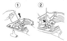
• Undo the screw in the centre of the pulley and remove the pulley. Insert and fasten a new starter cord to the pulley. Wind approx. 3 turns of the starter cord onto the pulley. Connect the pulley to the recoil spring so that the end of the spring engages in the pulley. Fit the screw in the center of the pulley. Insert the starter cord through the hole in the starter housing and the starter handle. Make a secure knot in the end of the starter cord.
