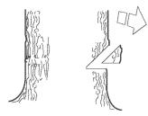
The directional cuts should run 1/4 of the diameter through the trunk and the angle between the top cut and bottom cut should be 45°.
