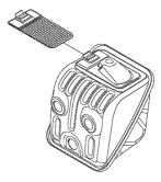
The muffler is designed to reduce the noise level and to direct the exhaust gases away from the operator. The exhaust gases are hot and can contain sparks, which may cause fire if directed against dry and combustible material.
