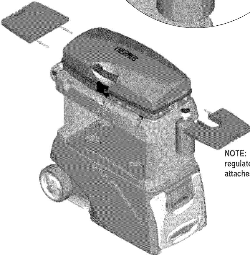
**NOTE:** Shelf with regulator cut-out attaches to right side.
