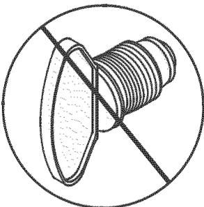
Use of this POL transport plug (plastic part with external threads) will defeat safety feature of valve.
