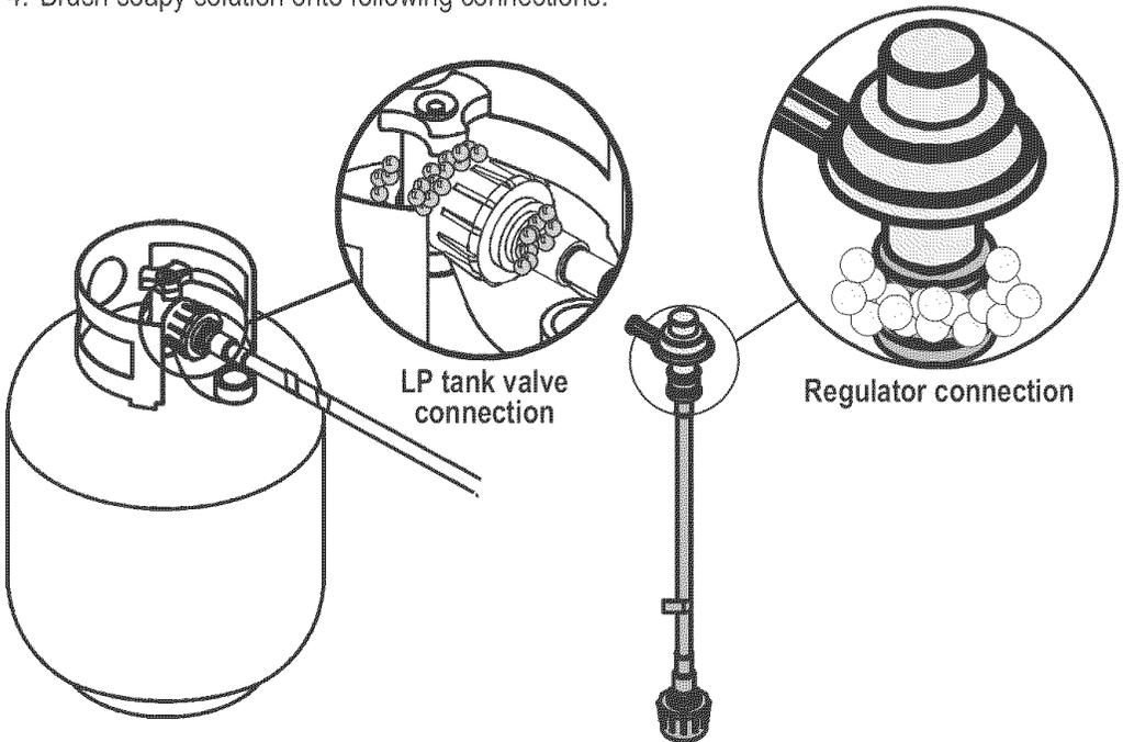
5. "If **growing**" bubbles appear, there is a leak. Close LP tank valve immediately and retighten connections. **If leaks cannot be stopped "do not try to repair"**. Call for replacement parts. Order new parts by giving the serial, model number and name of items needed to the Grill Service Center at 1-800-435-5194 U.S. or 1-800-387-6057 CAN.
