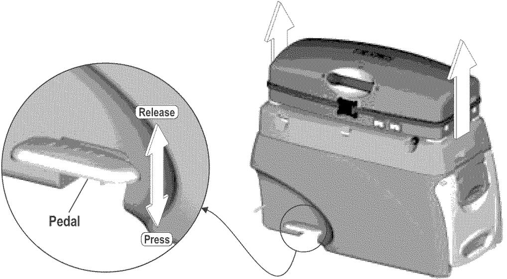
Slide cooler lid back to open and lift grill lid to remove packed components.
