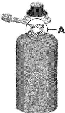
▲ If growing bubbles appear, there is a leak. Retighten connection and repeat steps 1 and 2
