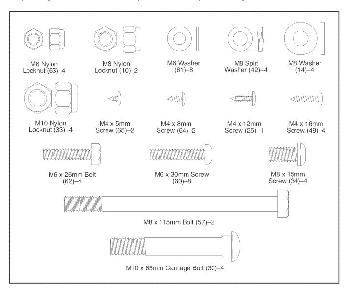
1. While another person lifts the front of the Frame (1) slightly, attach a Stabilizer (2) with two M10 x 65mm Carriage Bolts (30) and two M10 Nylon Locknuts (33).
