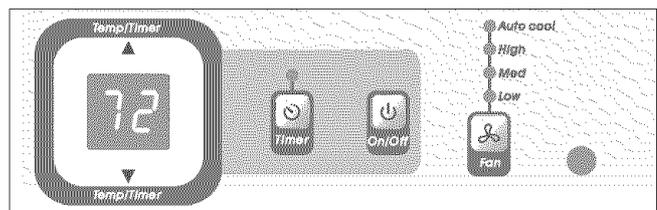
NOTE: Tap or hold either up (▲) or down (▼) button until the desired temperature is seen on the display. This temperature will be automatically maintained anywhere between 60°F (15°C) and 90°F (32°C). If you want the display to read the actual room temperature. See "To Operate on Fan Only" section on Page 7.
