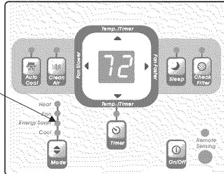
**NOTE:** In this mode, the fan will continue to run for 3 minutes after the compressor shuts off. The fan then cycles on for 2 minutes at 10 minute intervals until the room temperature is above the set temperature, at which time the compressor turns back on and cooling starts.
