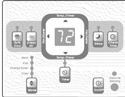
NOTE: Tap or hold either up (▲) or down (▼) button until the desired temperature is seen on the display. This temperature will be automatically maintained anywhere between 60°F (15°C) and 90°F (32°C). If you want the display to read the actual room temperature. See "To Operate on Fan Only" section on Page 7.
