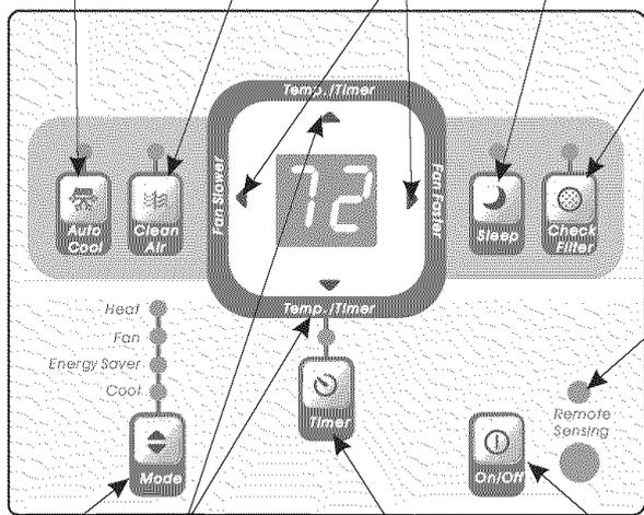
SETS MODE    ADJUSTS TEMPERATURE OR TIME    ACTIVATES TIMER    TURNS UNIT ON OR OFF
