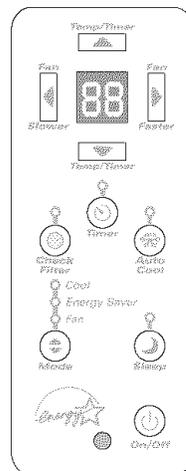
A 2 Digit Display is used to indicate the Fan Speed setting, from 10 through 99. When the "SLOWER" button is pressed the motor speed will slow down at multiple intervals (90 distinct settings), to a minimum setting of 10. To speed the motor up, press the "FASTER" button. The speed will increase at multiple intervals to a maximum setting of 99. After 5 seconds the control will automatically change back to displaying the set temperature.
