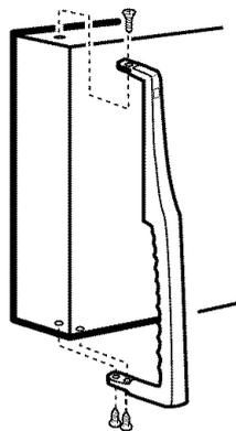
Move the plug button on the right side of the door to the handle screw hole on the left side.
