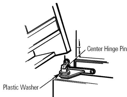
Lift the top hinge so the pin fits into the door socket. Support the door on the handle side and make sure the door is straight and the gap between the doors is even across the front. While holding the door in place, tighten the top hinge screws.
