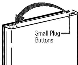
Move the large plug button from the left edge of the door and insert it into the hole on the opposite side.
