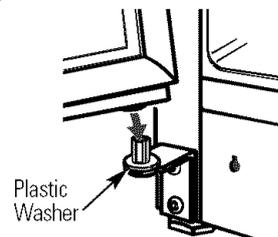
Straighten the door and line it up with the center hinge bracket.
