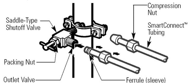
**NOTE:** Commonwealth of Massachusetts Plumbing Codes 248CMR shall be adhered to. Saddle valves are illegal and use is not permitted in Massachusetts. Consult with your licensed plumber.
