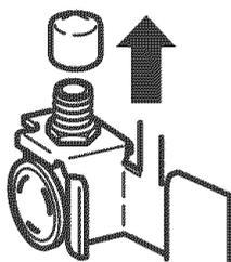
Insert the end of the tubing into the water valve connection as far as possible. While holding the tubing, tighten the fitting.
