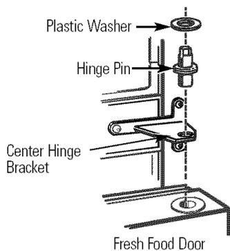
Remove the tape and tilt the door away from the cabinet. Remove and save the washer on the hinge pin. Lift the door straight up to free its bottom socket from the pin in the bottom hinge bracket.
