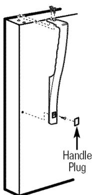
**After removing the handle:** Move the small plug buttons from the top right side of the door top and insert them into the holes on the opposite side.
