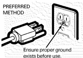
This appliance must be grounded. In the event of an electrical short circuit, grounding reduces the risk of electric shock by providing an escape wire for the electric current.
