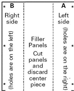
**C** Put together the panel assemblies. Remove the paper backing from the case side gasket and attach it to the angle. Push a pencil point through the gaskets to locate the holes in the angles.
