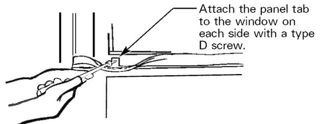
Attach the panel tab to the window on each side with a type D screw.
