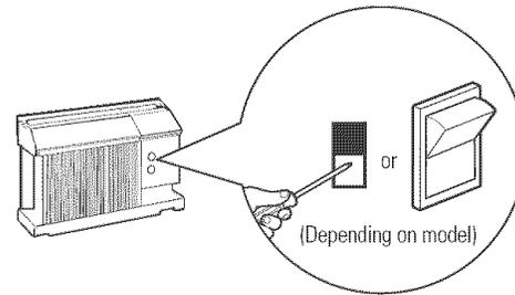
**Cool only models** have a rocker switch on the front of the control box.
