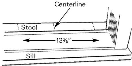
**B** Measure  $12\frac{3}{8}$ " from the centerline on both sides for the sill support brackets.
