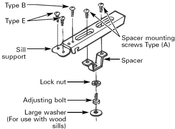
**C** Turn the bolts and tighten the lock nuts to make the sill supports level or tilt down  $1/8$ " to the outside. Line up the "V" notch with  $12\frac{3}{8}$ " marks. Drill pilot holes and attach the sill supports.
