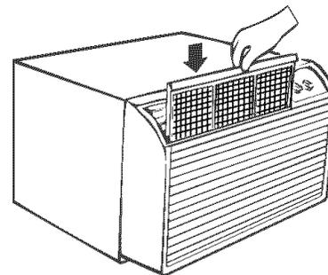
**▲ CAUTION:** Do not operate the air conditioner without the filter in place. If a filter becomes torn or damaged it should be replaced immediately.
