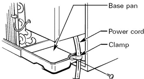
**C** When the wall outlet is to the left, extend the cord under the unit and hold it in place with the clamp.
