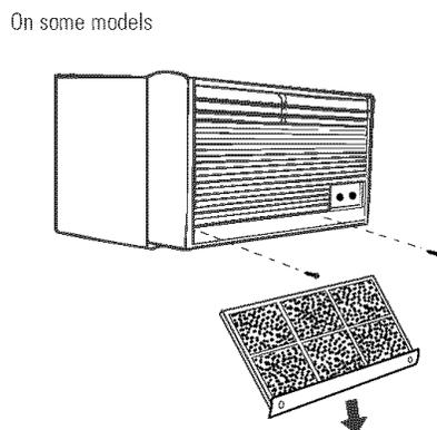
3. Pull the grille out from the bottom and lift up from the tabs on the top of the case.
