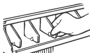
Remove the front grille to adjust the vertical louvers side-to-side to direct the air left or right.
