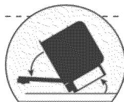
TIP: Pre-measure cabinet height to that of the dishwasher. Dishwasher should be 1/4" lower than that of the cabinet opening. It's easier to adjust the dishwasher outside the cabinet than inside.
