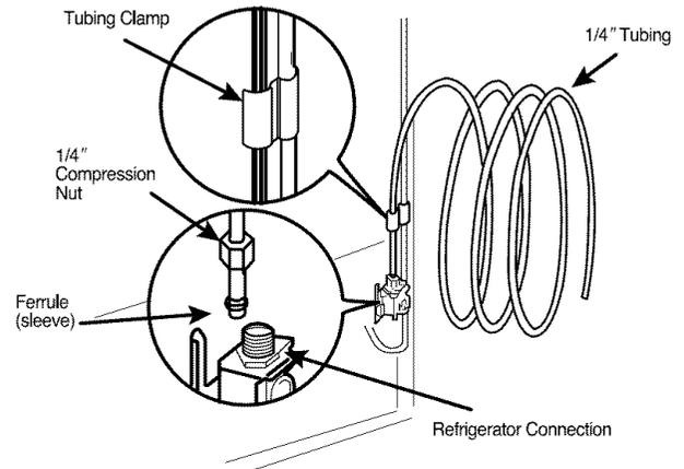
3. Insert the end of the copper tubing into the connection as far as possible. While holding the tubing, tighten the fitting.
