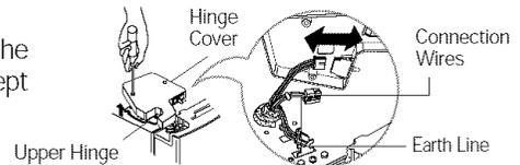
2) Remove the keeper by rotating it counter clockwise ① and then lifting the upper hinge up ②.
