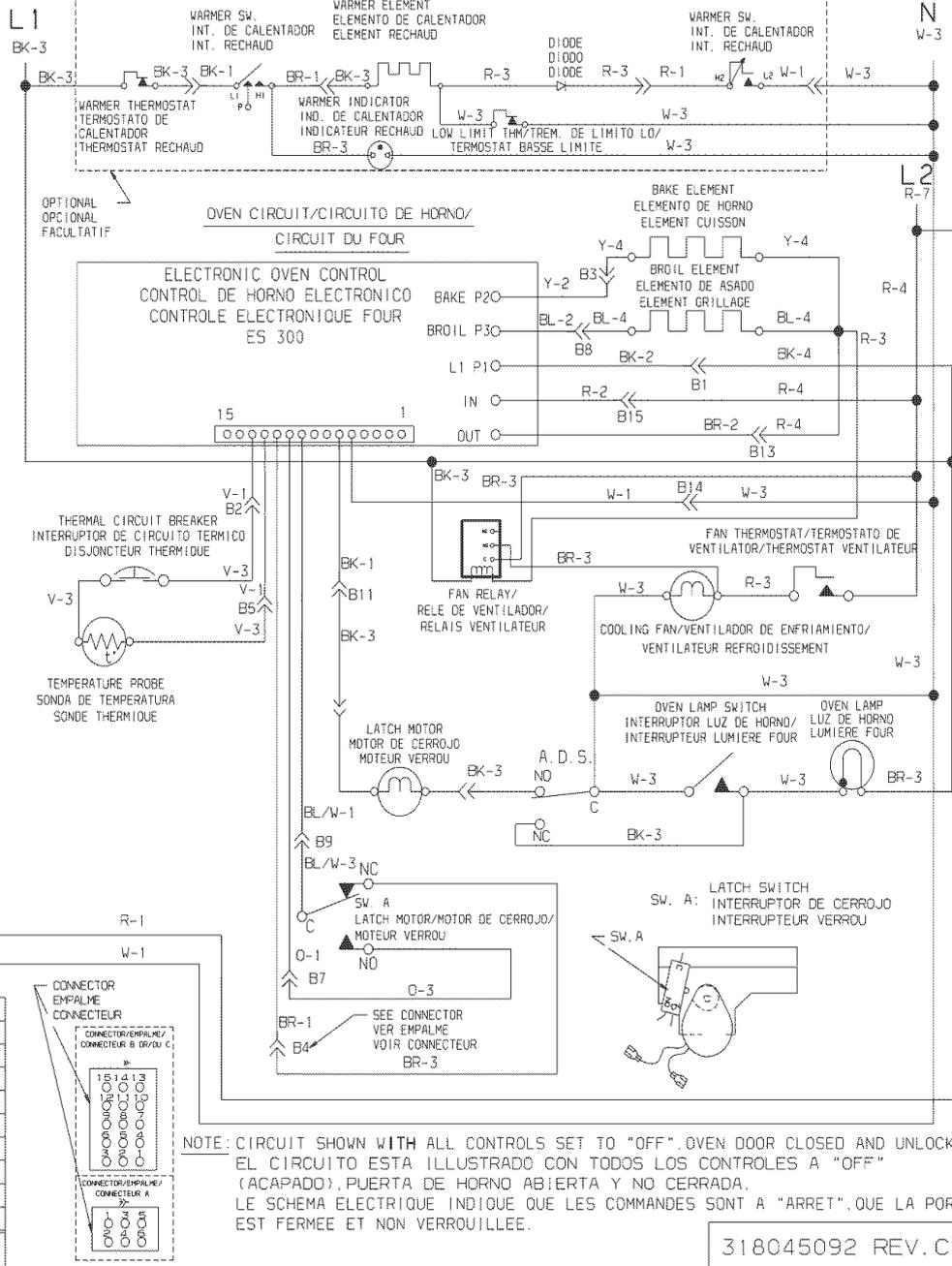
NOTE: CIRCUIT SHOWN WITH ALL CONTROLS SET TO "OFF". OVEN DOOR CLOSED AND UNLOCKED.
