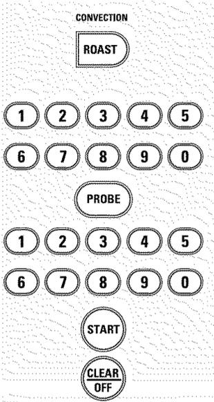
To change the oven temperature during the Convection Roast cycle, touch the **CONVECTION ROAST** pad and then touch the number pads to set the new desired temperature.
