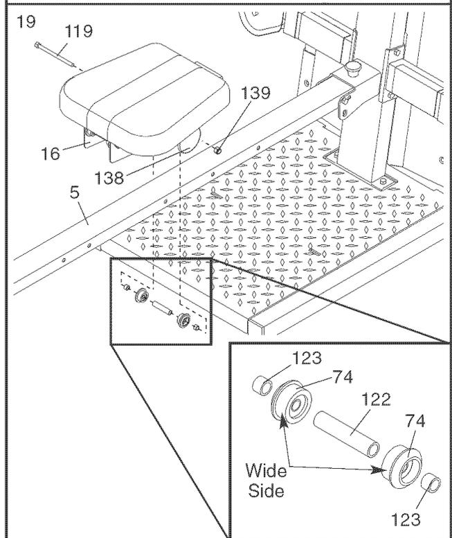
20. **Make sure that the wide sides of all six Seat Wheels (74) are pressed against the Rail (5).** While a second person presses down on the Seat (25), hold the bottom Seat Wheels firmly against the bottom of the Rail and properly tighten the indicated M8 Nylon Jamnut (139). **Do not over-tighten the Jamnut; the Wheels must be able to roll across the Rail.**
