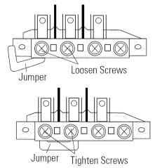
• Remove the jumper and place between the first and second screws, tighten the screws to hold the jumper.
