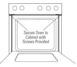
Secure oven to cabinet with screws provided. Single ovens use 2 screws, one on each side. Double ovens use 4 screws, 2 on each side.
