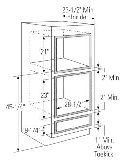
**NOTE:** The middle rail separating the two openings may need to be larger than the 2" minimum shown. Always refer to the individual installation instructions packed with each product for specific requirements.
