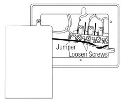
Loosen the first and second screws in the terminal block as shown.
