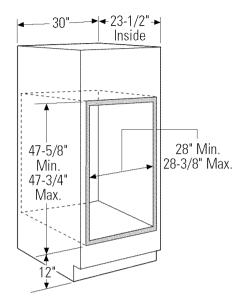
Order a 30" oven cabinet with the cutout sized to fit the double oven.
