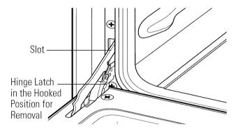
• Close the door about half way, or to a 45° opening. Pull the door straight off and away from the oven.
