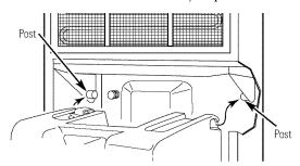
Make sure the bucket is locked securely in place by pressing down on the upper back edge of the bucket. It will be firmly seated when properly installed.
