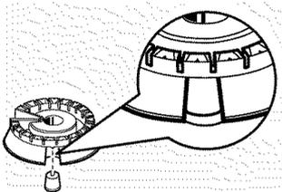
Make sure the slot in the burner head is positioned over electrode.
