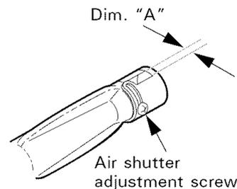
5. Check the inner cone of the flame. It should be between  $1/2$ " and  $3/4$ " long for the oven bake and broil burners.
