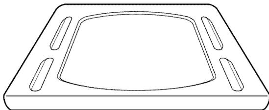
4. Remove the four screws holding the burner baffle (flame spreader) to the burner box.
