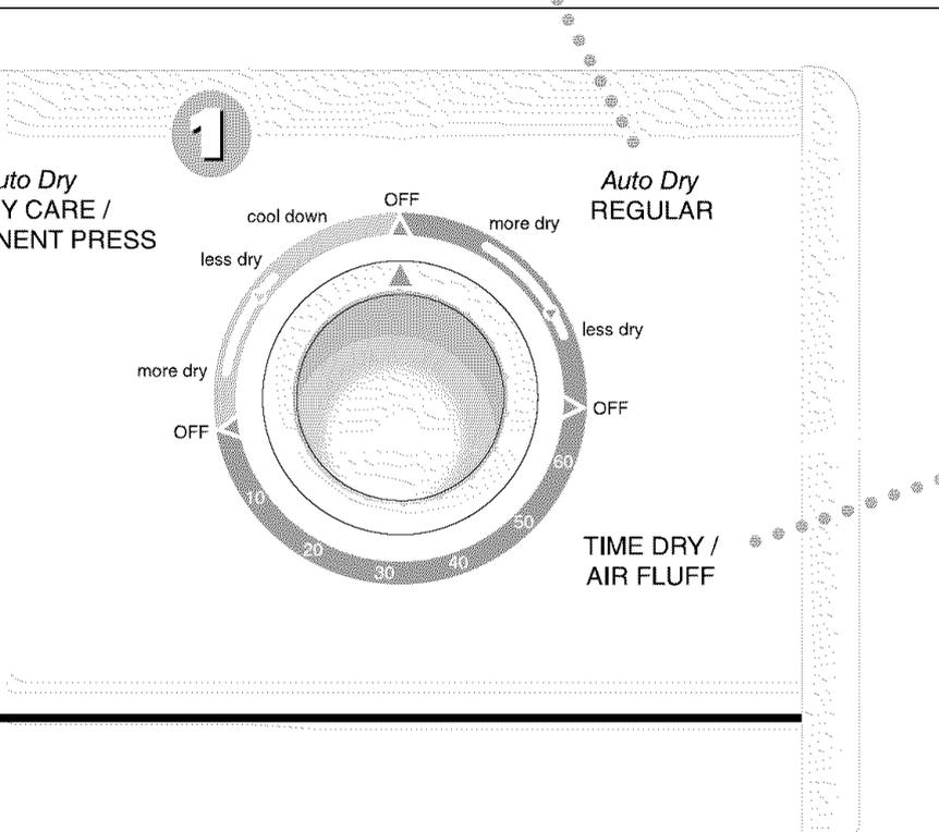
**TIME DRY/AIR FLUFF** may be selected for any load if the *Auto Dry* sensor system is not desired. Set the control to the desired number of minutes. Set the appropriate heat for drying by rotating the temperature knob.
