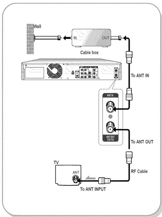
**Method 3 : Antenna + TWIN TRAY DVD RECORDER + Cable box + TV : Cable box with a few scrambled channels**
