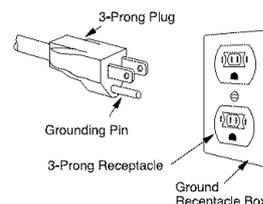
The Power Supply Cord and plug must be connected to a separate 120 Volt AC, 60 Hz, 15 Amp, or more branch circuit, single grounded receptacle. The receptacle should be located inside the cabinet directly above the Microwave Oven mounting location as shown in Figure 2.
