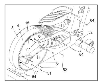
Next, remove the four Screws (51) from the right Pedal Disc (15), and slide the Pedal Disc off. Remove all Screws (52, 64) from the Right Side Shield (4) and the two Screws (77) from beneath the Pedal Disc, and remove the Right Side Shield (4). Remove all Screws (52) from the Left Side Shield (3) and remove the Left Side Shield.
