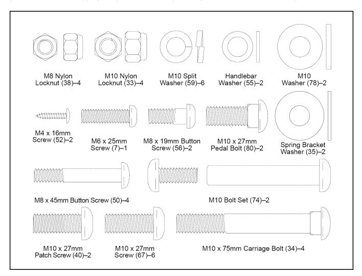
Identify the Front Stabilizer (10), which has Wheels (22) attached to it. While another person lifts the front of the Frame (1), attach the Front Stabilizer to the Frame with two M10 x 75mm Carriage Bolts (34) and two M10 Nylon Locknuts (33). Make sure that the Front Stabilizer is turned so the Wheels are not touching the floor.
