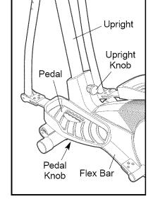
counterclockwise a few turns to loosen it. Next, pull the knob, raise or lower the upright to the desired height, and then release the knob. Move the upright up and down slightly until the pin on the knob snaps into one of the four adjustment holes in the upright. Make sure that the upright is not resting on top of the pin. Then, turn the knob clockwise until it is tight.
