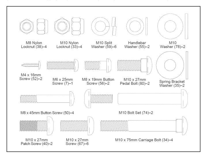
1. Identify the Front Stabilizer (10), which has Wheels (22) attached to it. While another person lifts the front of the Frame (1), attach the Front Stabilizer to the Frame with two M10 x 75mm Carriage Bolts (34) and two M10 Nylon Locknuts (33). Make sure that the Front Stabilizer is turned so the Wheels are not touching the floor.
