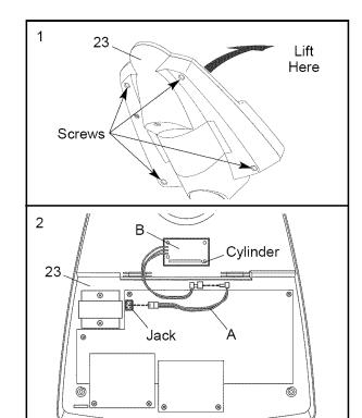
2. Plug the short jumper wire (A) into the indicated jack on the Console (23). Connect the other end of the short jumper wire to the wire on the receiver (B). Note: The included long jumper wire is not needed.
