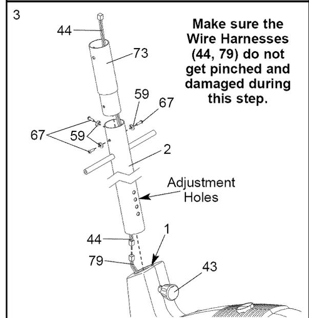
Next, turn the Upright Knob (43) counterclockwise several turns. Pull the Knob, slide the Upright (2) down until the Knob is aligned with one of the four adjustment holes, and then release the Knob. Do not tighten the Knob yet.
