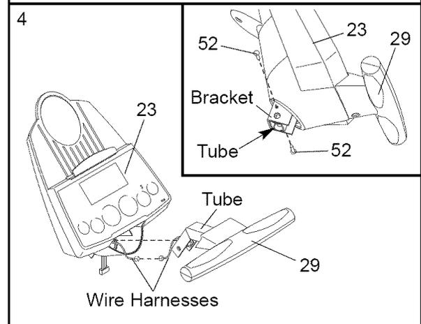
Refer to the inset drawing. Align the holes in the bracket on the Console (23) with the holes in the metal tube on the Handgrip Pulse Sensor (29). Tighten two M4 x 16mm Screws (52) through the bracket into the tube as shown.
