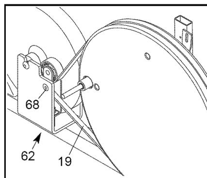
Next, loosen the M8 x 22mm Flat Head Screw (68) and turn the M10 x 70mm Bolt (62) until the Drive Belt (19) is tight. When the Drive Belt is tight, tighten the Flat Head Screw. Reattach the side shields.
