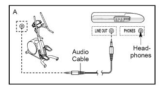
B. Plug one end of the audio cable into the jack beneath the console of the stepper. Plug the other end of the cable into a 3.5mm Y-adapter (available at electronics stores). Plug the Y-adapter into the PHONES jack on your CD player. Plug your headphones into the other side of the Y-adapter.
