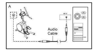
B. Plug one end of the audio cable into the jack beneath the console of the stepper. Plug the other end of the cable into a 3.5mm Y-adapter (available at electronics stores). Plug the Y-adapter into the PHONES jack on your computer. Plug your headphones or speakers into the other side of the Yadapter.
