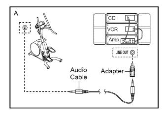
B. Plug one end of the audio cable into the jack beneath the console of the stepper. Plug the other end of the cable into the included adapter. Plug the adapter into an RCA Y-adapter (available at electronics stores). Next, remove the wire that is currently plugged into the LINE OUT jack on your stereo and plug the wire into the unused side of the Y-adapter. Plug the Y-adapter into the LINE OUT jack on your stereo.
