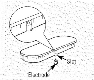
Make sure the slot in the burner head is positioned over the electrode. Use a sewing needle or twist-tie to unplug the small hole in the burner head.
