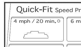
When a program is selected, the Speed display will flash the maximum speed setting of the program for a few seconds, the Time/Pace display will show how long the program will last, and the matrix will show the first seven speed settings of the program.
