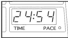
To reset the displays, press the Stop button, remove the key, and then reinser the key.
