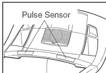
will be shown. For the most accurate heart rate reading, continue to hold the contacts for about 15 seconds.
