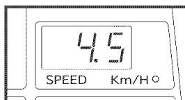
Speed buttons. Each time a button is pressed, the speed setting will change by 0.1 mph; if a button is held down, the speed setting will change in increments of 0.5 mph. **Note: The console can display speed and distance in either miles or kilometers. For simplicity, all instructions in this section refer to miles.**
