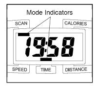
mode indicator will show which mode is currently displayed. Note: If you have selected a different mode, repeatedly press the Mode button to reselect the scan mode.
