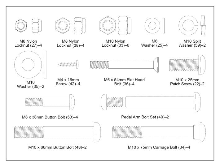
1. Identify the Front Stabilizer (10), which is narrower than the Rear Stabilizer (not shown). While another person lifts the front of the Frame (1), attach the Front Stabilizer to the Frame with two M10 x 75mm Carriage Bolts (34) and two M10 Nylon Locknuts (33).
