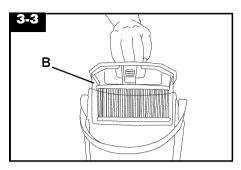
Remove filter chamber (B) from dirt cup.
