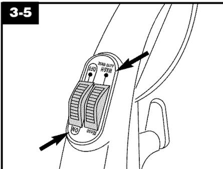
7. Squeeze trigger to release cleaning solution and **slowly** push deep cleaner forward (equals one wet stroke).
