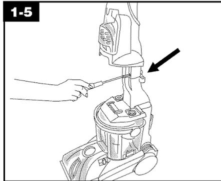
Push **bolts** into holes on **front of handle**. If **bolts will not go through hole easily, handle is not pushed completely down**. Place **nuts** in recessed areas on **back of the handle**. Hold each nut in place while tightening each bolt securely (from the front of the handle) with a Phillips screw driver.
