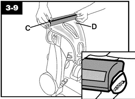
2. With foam strip (C) (located under the netting) in position as shown, place attachment on front of nozzle (D).
