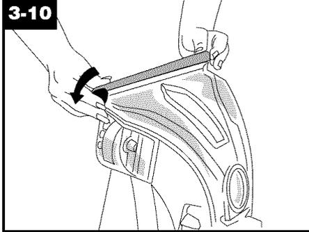
3. Push attachment against nozzle while rotating attachment downward until both ends snap into place.
