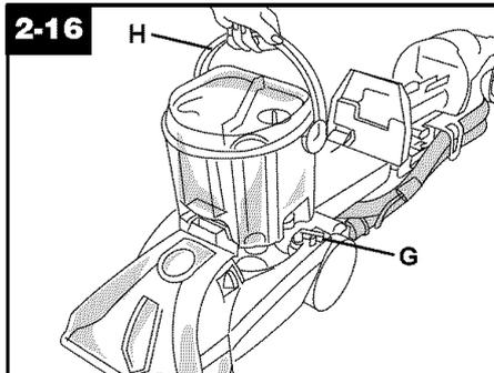
Turn recovery tank latches (G) outward (one on each side of tank).
