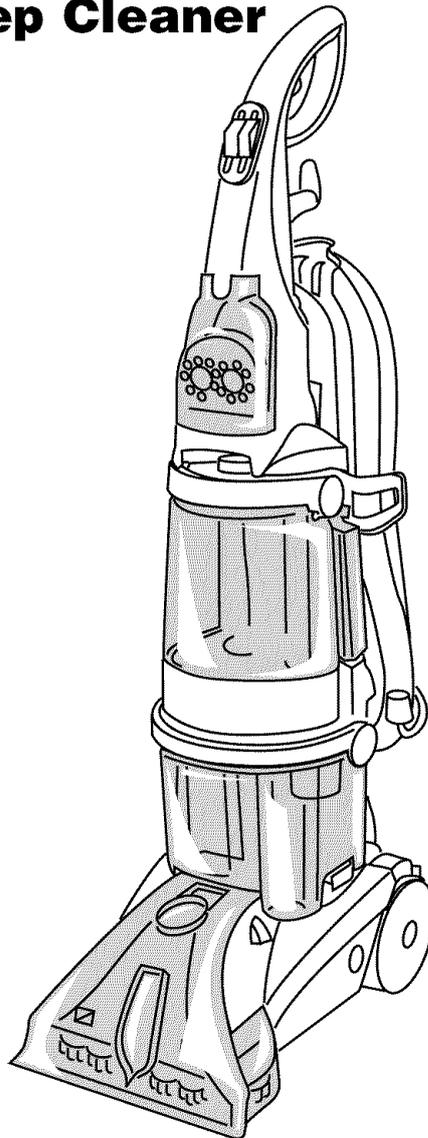
**SteamVac™ V2™ Deep Cleaner cleans carpet fibers by applying hot tap water and cleaning solution.**
