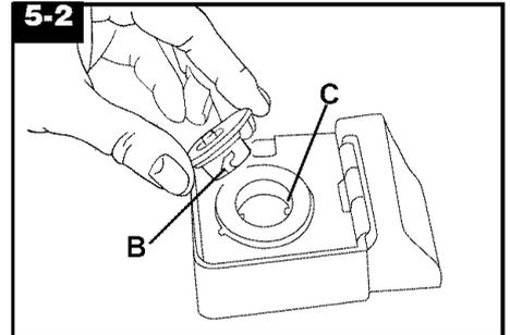
3. Align slots (B) on cap with tabs (C) in opening.
