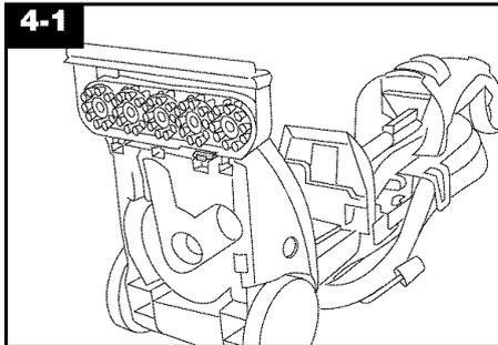
With handle in upright position, tilt cleaner back until handle rests on the floor.
