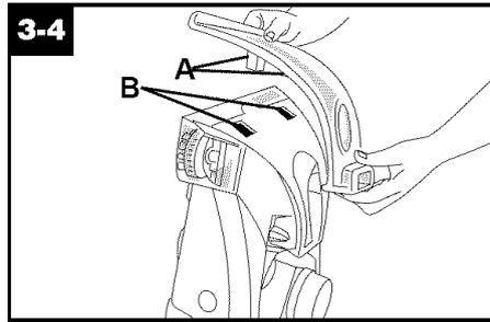
To replace nozzle, line up tabs (A) on nozzle with holes (B) in cleaner. Slide tabs into holes.
