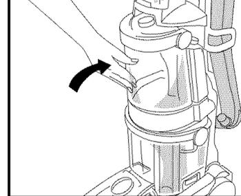
Position bottom of tank onto cleaner and pivot tank to snap it into place.
