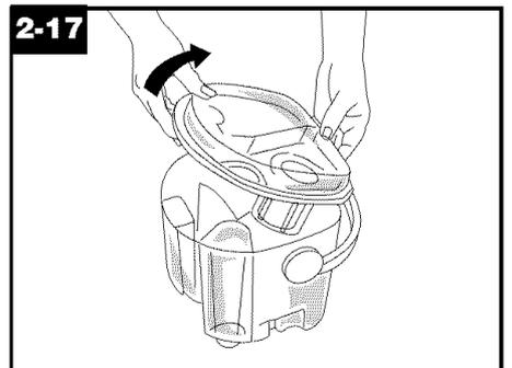
Lower handle toward back of tank to unlock lid. Lift lid off tank.
