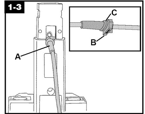
**NOTE:** If the cord protector (A) on back of handle should become dislodged during unpacking, **make sure it is repositioned properly before continuing with assembly** of your deep cleaner. With the arrow (B) on the cord protector pointing down, press groove (C) in the cord protector into slot in the lower handle.
