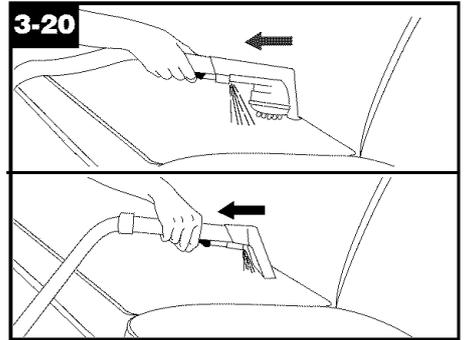
8. Gently press the tool onto the fabric. Press the trigger and slowly pull the nozzle over the fabric.
