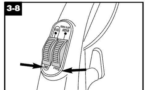
11. If you would like to rinse the carpet with water only, set Rinse Setting switch to **RINSE** (Fig. 3-8). Repeat steps 7-9. In this setting, rinsing will be done on both forward and reverse strokes.
