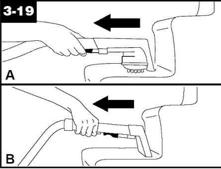
11. Lift tool, and position it against riser. Pull tool **slowly** over carpet without pressing trigger (dry stroke).
