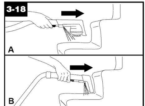
9. Pre-spray the carpeted stair by holding the tool (A) or (B) about one inch above the carpet and push it forward while pressing the trigger (equals one wet stroke).
