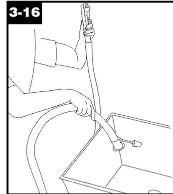
Drain solution tube by placing round end in sink and raising nozzle above your head. Press the trigger.
