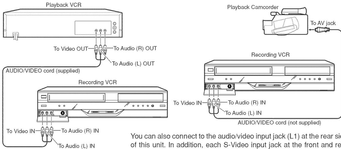
You can also connect to the audio/video input jack (L1) at the rear side of this unit. In addition, each S-Video input jack at the front and rear sides can be used for recording on the disc. (The S-Video input jack cannot be used for recording on the video tape.)
