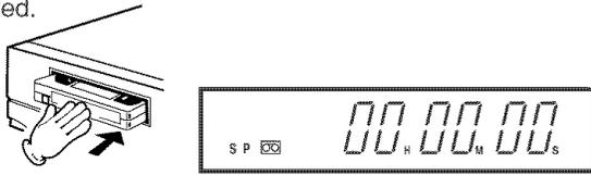
Insert the cassette tape with its labeled side facing up and the erase prevention tab positioned at your left. An inverted cassette tape cannot be inserted.
