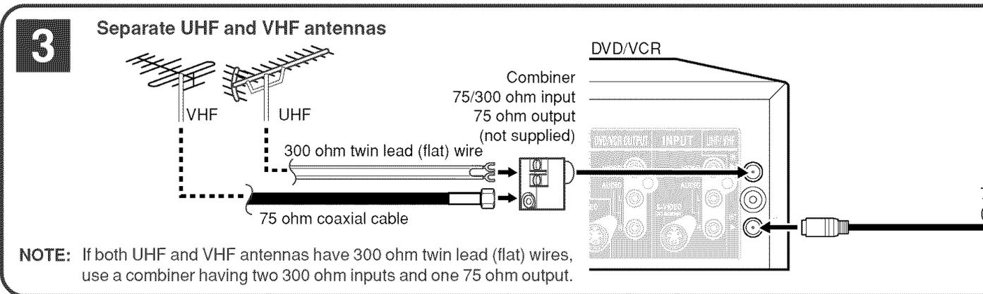
**NOTE:** If both UHF and VHF antennas have 300 ohm twin lead (flat) wires, use a combiner having two 300 ohm inputs and one 75 ohm output.
