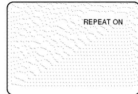
3 When "REPEAT ON" is selected, the tape is played back to the end, and then, it is automatically rewound to the starting point and played back again. The display "REPEAT ON" goes out in about 3 seconds.
