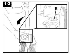
Press upper handle release button (B) back to fold handle to storage position.
