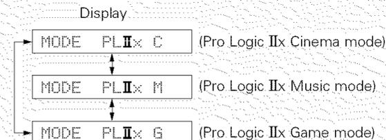
※ When the "SB CH. OUT" parameter is set to "OFF". (Set "S. BACK" at system setup to "NONE".)
