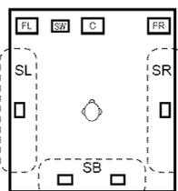
In this case it is important to achieve the same sense of expansion as in a movie theater with the surround channels. To do so, in some cases the number of surround speakers is increased (to four or eight) or speakers with bipolar or dipolar properties are used.
