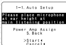
3 Press the **CURSOR**  $\Delta$  or  $\nabla$  button to select "Power Amp Assign", then press the **CURSOR**  $\triangleleft$  or  $\triangleright$  button to select "S. Back", "ZONE2" or "Bi-Amp".
