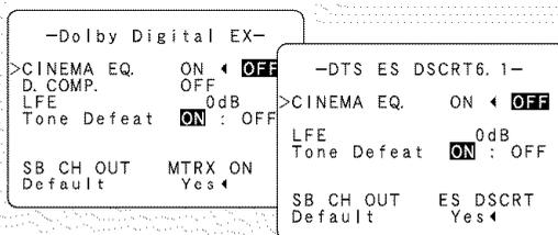
**6** Press the **SURROUND PARAMETER** button, and press the **CURSOR**  $\Delta$  or  $\nabla$  button to select the various parameters.
