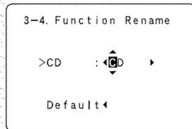
**3** Press the **CURSOR**  $\triangleleft$  or  $\triangleright$  button to move the cursor (■) to the character, number, symbol or punctuation mark you wish to input, and press the **CURSOR**  $\Delta$  or  $\nabla$  button to select that character.
