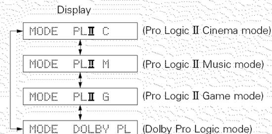
**5** Press the **SURROUND PARAMETER** button, and press the **CURSOR** ▲ or ▼ button to select the various parameters.
