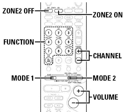
**Outputting a program source to amplifier, etc., in a different room (ZONE2 mode)**
