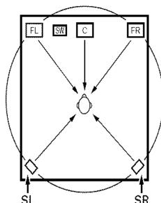
In this case the speakers should surround the listener from all sides to create a uniform sound field from 360°. Ideally the surround speakers should function as “point” sound sources in the same way as the front speakers.
