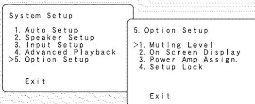
**2** Press the **CURSOR**  $\Delta$  or  $\nabla$  button to select “Muting Level” at the “Option Setup” menu, then press the **ENTER** button.
