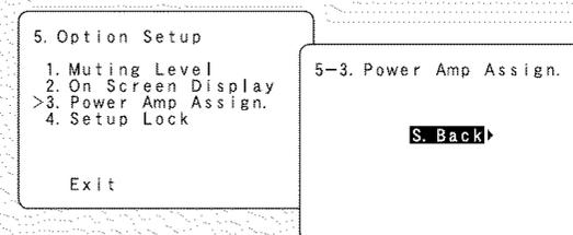
**2** Press the **CURSOR**  $\triangleleft$  or  $\triangleright$  button to select the Amp Assign mode according to the speaker system you want to set up.
