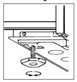
For good baking results, your range should be level and rest firmly on a level floor. Screw type levelling legs are provided at each corner of the range at the base. Remove the storage drawer to adjust the leveling legs.
