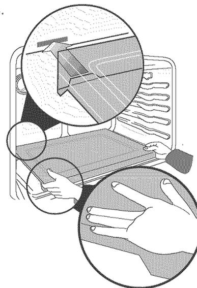
Grasp the oven bottom by the front corner on each side to raise and lower the oven bottom.
