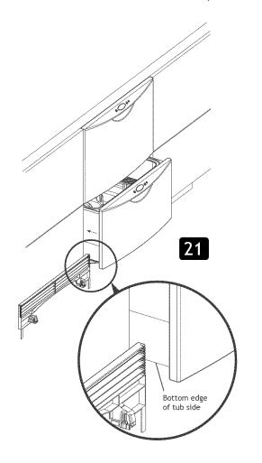
Partially open the bottom drawer. Turn Prefinished Toe Kick upside down and hold vertically against the bottom edge of the *Tub side* (not the drawer front).
