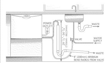
**OPTION 1**DishDrawer® and Standpipe Ø11/2" (38mm) with Air Gap.
