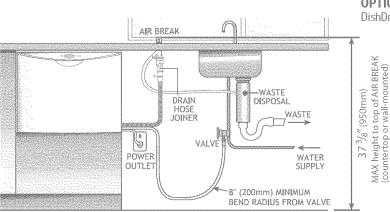
$\begin{array}{l} \textbf{OPTION 3} \\ \textbf{DishDrawer} \\ \textbf{®} \ \textbf{using Air Break with Drain Hose Joiner.} \end{array}$
