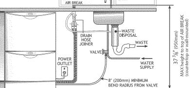
$\label{eq:DishDrawer} \textbf{$\mathbb{R}$ using Air Break with Drain Hose Joiner.}$
