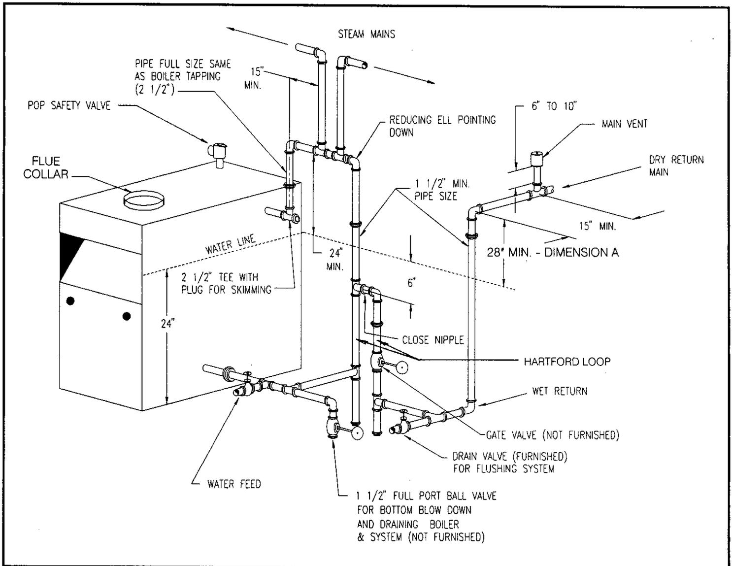
5. For installers choosing to use both supply tappings, Figure 6A shows the **correct** way to pipe this system. Figure 6B shows the **wrong** way to pipe a header with two risers.
