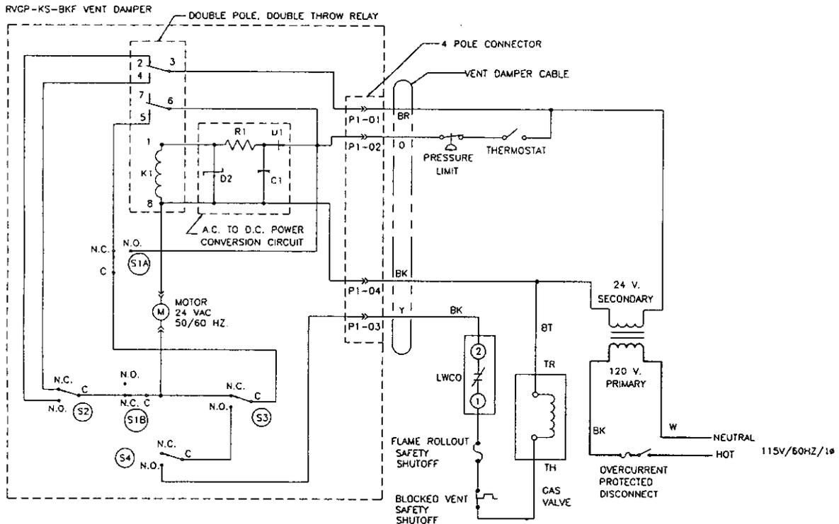
**IF ANY OF THE ORIGINAL WIRE AS SUPPLIED WITH THIS APPLIANCE MUST BE REPLACED, IT MUST BE REPLACED WITH TYPE 105° C THERMOPLASTIC WIRE OR ITS EQUIVALENT.**
