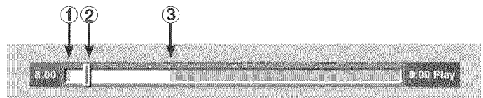
Figure 14. TV Pause slider. 1. Limit of backward scan. 2. Current viewing point in recorded portion of program. 3. Current broadcast point (limit of forward scan)
