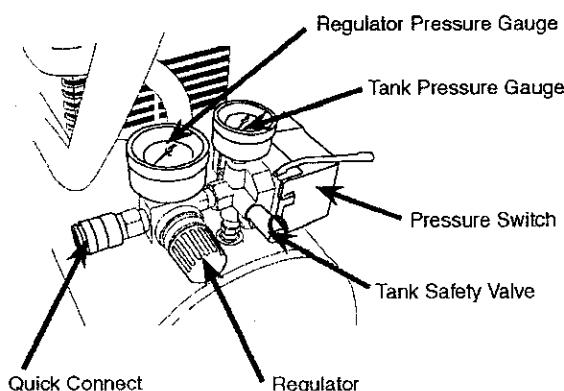
**Cut-Out Pressure:** The point at which the motor stops when the tank has reached maximum air pressure.
