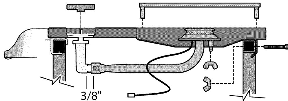
**Hook Electrode wire to side terminal on igniter.**
