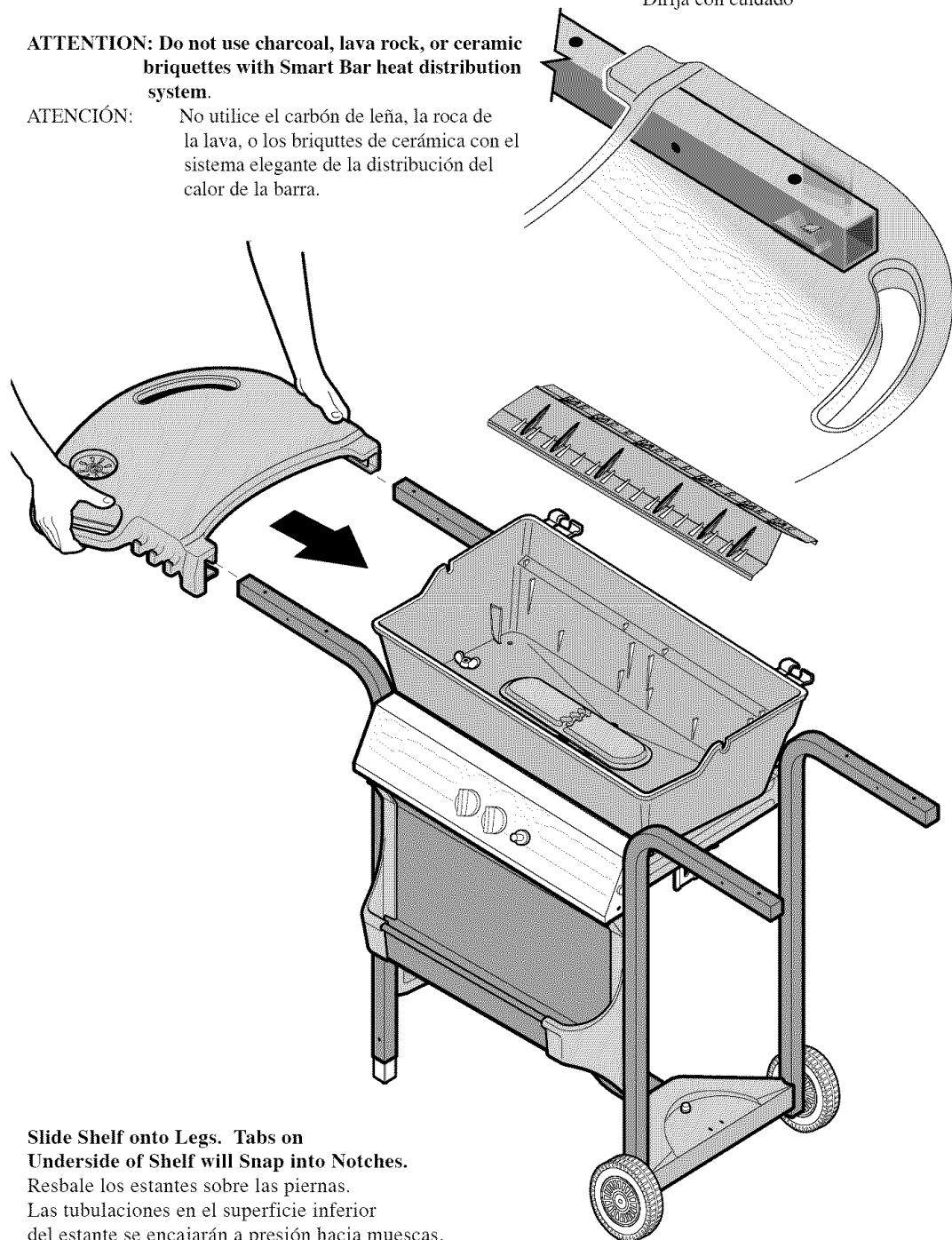
**Slide Shelf onto Legs. Tabs on Underside of Shelf will Snap into Notches.**
