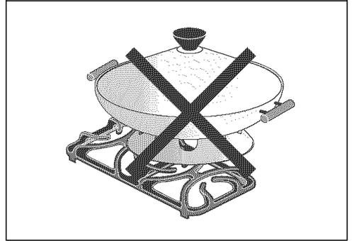
**Wire trivets:** Do not use wire trivets. Cookware bottoms must be in direct contact with the grates.
