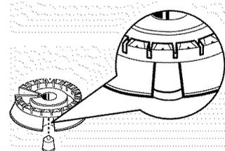
Replace the matching size caps onto the heads. There is one large, two small and two medium caps.
