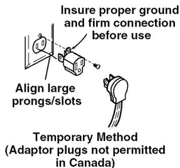
**CAUTION:** Attaching the adaptor ground terminal to the wall receptacle cover screw does not ground the appliance unless the screw is metal, and not insulated, and the wall receptacle is grounded through the house wiring. The customer should have the circuit checked by a qualified electrician to make sure the receptacle is properly grounded.
