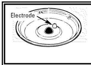
The electrode of the spark igniter is exposed when the burner head is removed. When one burner is turned to **LITE**, all the burners spark. Do not attempt to disassemble or clean around any burner while another burner is on. An electric shock may result, which could cause you to knock over hot cookware.
