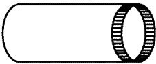
Broan Model 407 Straight Duct 7-in. round x 2-ft. long Equivalent length 2 ft.
