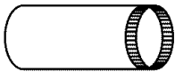
Broan Model 406 Straight Duct 6-in. round x 2-ft. long Equivalent length 2 ft.
