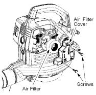
A dirty air filter decreases engine performance and increases fuel consumption and harmful emissions. Always clean after every 5 hours of operation.
