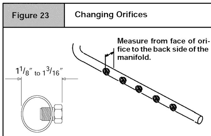
5. Reinstall manifold. Ensure burners do **NOT** bind on new orifices.
