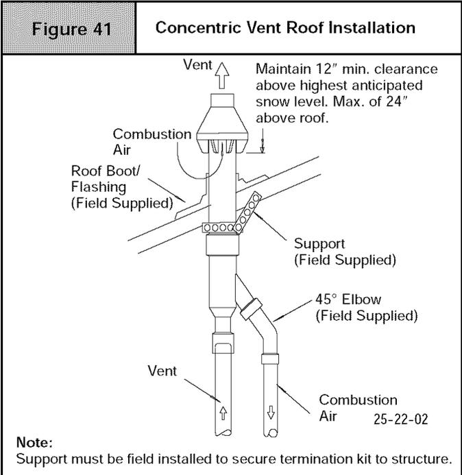
3. Cut one 5" diameter hole through the structure for the NAHA001CV Kit or one 4" diameter hole for the NAHA002CV Kit .
