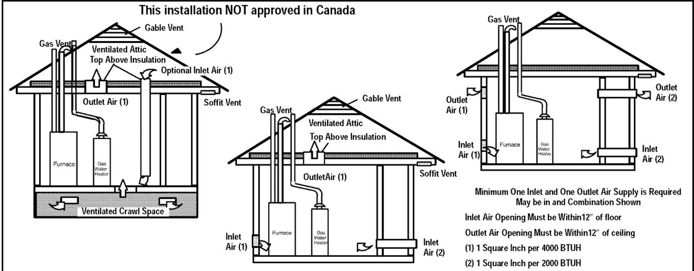
3. One opening **MUST** be within 12" of the floor and the second opening within 12" of the ceiling.
