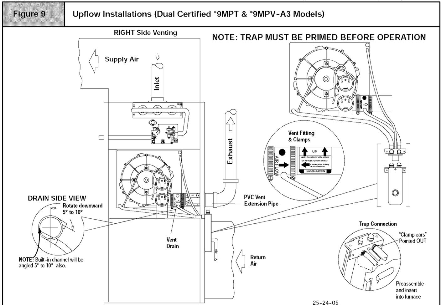
For left or right side mounted condensate trap, the pressure tap on the condensate trap **MUST** be connected to the unused pressure tap located on the upper right hand corner of the plastic transition box. Remove the plastic caps from the pressure taps on the condensate trap and the plastic transition and connect with the 5/16" OD rubber hose. (See **Figure 8** and **Figure 9**)
